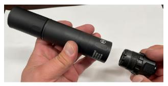
\*When using this suppressor on a weapon system with a fixed barrel, it must be used with the direct thread mount (pictured below). If the suppressor is shot with the booster assembly on a fixed barrel system, it will damage the booster assembly or even the suppressor. Replace the booster assembly with the provided direct thread mount when using this suppressor on a fixed barrel system.
