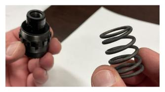
Apply grease on the 0-ring inside the booster cap. Thread on the booster cap, snug firmly by hand.
