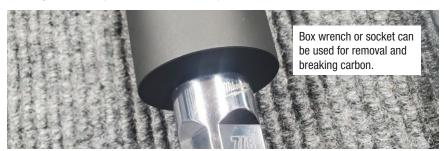
NOTE: Use a torque wrench only for installing, not when removing, as this can damage the torque wrench.
