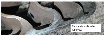
As shown below: turning the suppressor tube assembly over the monocore to break free any carbon deposits.
