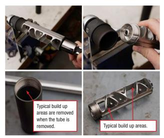
When fully cleaned, the interior of the tube will still have visible carbon deposits. It will not be possible to get all of them off. The best way to clean the carbon off of the interior of the tube is to turn the tube around the MonoKore. Unthreading the suppressor tube and removing the tube from the mount and core assembly should remove most of the carbon deposits that need attention.
