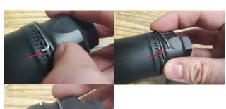
Remove the spring and set it aside until after the cleaning and maintenance is completed.
