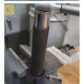
Place the provided DSX-M assembly tool in a vice securely.
