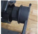
In case a 1" wrench cannot reach the primary tool feature, use a common screwdriver across both cuts, and unthread the direct thread mount.
