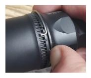
Using anything non-metallic, even a fingernail, push the straight end of the spring in the groove. This will cause a portion of the spring to lift up. With the other hand, use the same tool to pick the bent portion of the spring and lift it out of its groove
