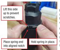
Place the straight end of the spring in the spring groove. Hold that end in place in the groove with a thumb or finger.
