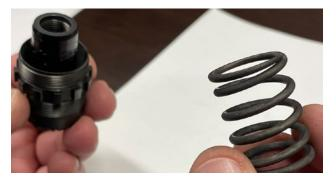
Insert the booster spring into the booster body.
