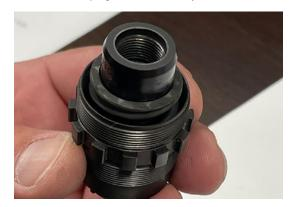
Apply grease on the 0-ring inside the booster cap. Thread on the booster cap, snug firmly by hand.
