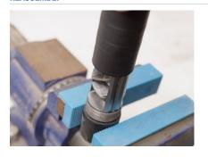
After the suppressor has been cleaned / serviced it may be reassembled. In order to reassemble the suppressor, hold the suppressor in the same way as it was held during disassembly.
