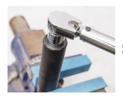
With a torque wrench and a 7/8" socket, torque the suppressor tube to the mount at 25 ft\*lbs.
