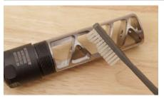
When fully cleaned, the interior of the tube will still have visible carbon deposits. It will not be possible to get all of them off. The best way to clean the carbon off of the interior of the tube is to turn the tube around the MonoKore. Unthreading the suppressor tube and removing the tube from the mount and core assembly should remove most of the carbon deposits that need attention.
