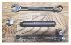
The suppressor tube is torqued to the mount and red (permanent) Loctite® is used to bind them together. If there is a problem, return the suppressor to the factory where experienced technicians can separate and replace these components.
