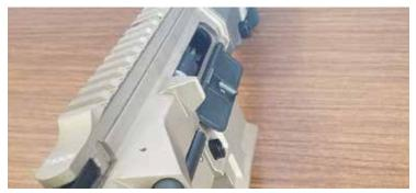
**5.** Press bottom of bolt catch and allow bolt to move forward until it engages bolt catch.
