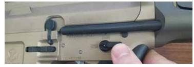
**3.** Remove magazine from magazine well by depressing the magazine release and extracting the magazine from the magazine well.
