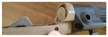
**NOTE:** For the PDX model, place buffer into rear of bolt carrier. Ensure buffer is fully seated.
