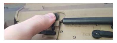
**5.** Tap forward assist to ensure bolt is fully seated forward.
