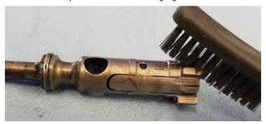
**CAUTION: DO NOT** use wire brush or any other type of abrasive material when cleaning aluminum surfaces.
