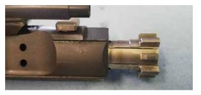
8. Insert firing pin retaining pin.
