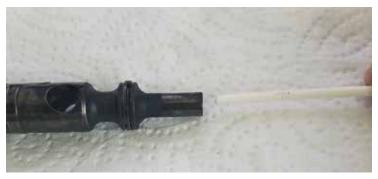
4. Clean firing pin hole with pipe cleaner or swab.
