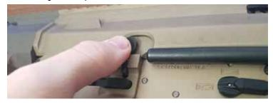
Alternatively, the bolt catch can be engaged by pulling the charging handle fully rearward and depressing the bottom portion of the bolt catch / release. Push the charging handle forward.
