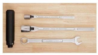
The tools required to assemble, disassemble, and maintain the PRS:30 are the a 1" wrench or socket (mount), a 1  $\frac{1}{4}$ " wrench or socket (tube), and a 7/8" wrench or socket (MonoKore).
