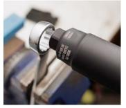
To disassemble the PRS:30, begin by securing the 1" socket and driver or wrench in a vice, as shown. This will serve as the holding point for the mount portion of the suppressor.
