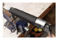
Using a driver and a 1 ¼" socket or a 1 ¼" wrench, unthread the suppressor tube. It will take some force to unthread the suppressor tube. If the tube seems very hard to remove, you may put some solvent or oil into the suppressor in order to aid disassembly. This may happen if the suppressor has not been maintained properly. Maintaining the suppressor often will prevent this from happening for the most part.
