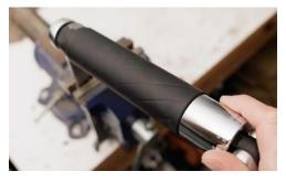
When assembly is completed the suppressor is ready to be used again. The PRS:30 should be maintained in this way each time after a range day if possible. If the PRS:30 is not at a minimum disassembled in the described way between range days, carbon deposits can build up on the interior surfaces of the suppressor and harden making disassembly progressively more difficult.
