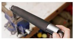
Using a driver and a 1  $\frac{1}{4}$ " socket or a 1  $\frac{1}{4}$ " wrench, unthread the suppressor tube. It will take some force to unthread the suppressor tube. If the tube seems very hard to remove, you may put some solvent or oil into the suppressor in order to aid disassembly. This may happen if the suppressor has not been maintained properly. Maintaining the suppressor often will prevent this from happening for the most part.
