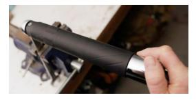
When assembly is completed the suppressor is ready to be used again. The PRS338 should be maintained in this way each time after a range day if possible. If the PRS338 is not at a minimum disassembled in the described way between range days, carbon deposits can build up on the interior surfaces of the suppressor and harden making disassembly progressively more difficult.
