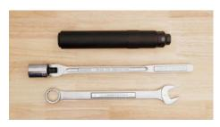
The tools required to assemble, disassemble, and maintain the PRS338 are a 1" wrench or socket (mount) and 1  $\frac{1}{4}$ " wrench or socket (tube).
