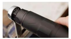
To disassemble the PRS338, begin by securing the 1" socket and driver or wrench in a vice, as shown. This will serve as the holding point for the mount portion of the suppressor.
