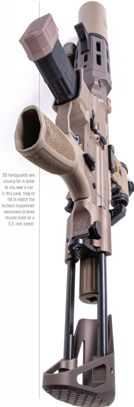
SD handguards are usually fat in order to slip over a can. In this case, they're fat to match the bulbous suppressor necessary to tame muzzle blast on a 5.5-inch barrel.
