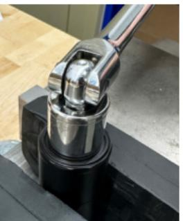
Began by first Placing the MS45 in a soft jaw vice, then taking a 3/4 socket wrench unscrew the end cap from the suppressor.
