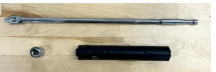
The tools required to assemble, disassemble, and maintain the MS-45 are a 3/4 socket wrench.
