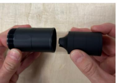
Remove baffle stacks from the front module.
