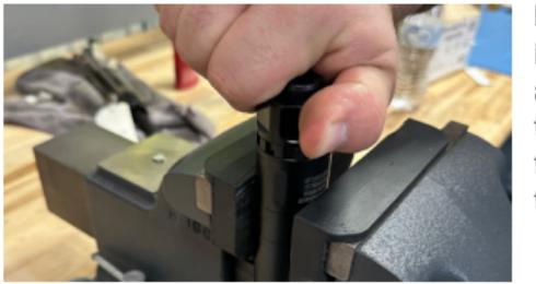
Flip the Suppressor in the soft jaw vice and unscrew by hand the booster system from the suppressor tube.
