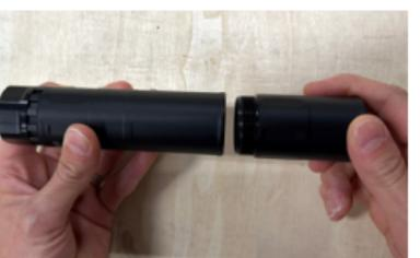
By hand unscrew the front module from suppressor.
