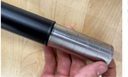
Remove baffle stacks from the main body module.
