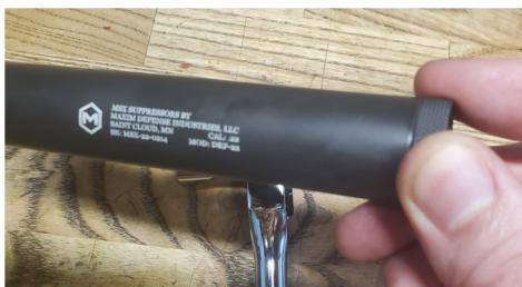
The suppressor MonoKore is threaded into the suppressor tube. The threads are standard right-hand threads. The threaded end of the suppressor MonoKore has a knurled portion to ease removal and installation for maintenance.
