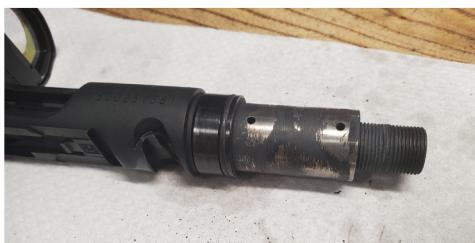
Once the barrel is unthreaded, the rear portion of the tube assembly and the barrel may be cleaned with a firearms solvent or oil of your choice. Using a brush or rag, clean the barrel assembly components shown. Do no remove the diffuser from the barrel assembly.
