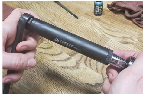
If the MonoKore is stuck within the tube, the front of the MonoKore is a tool feature that fits a 1/2" socket and the rear of the suppressor has a 3/4" socket feature. If further leverage is needed please contact Maxim Defense Customer Support.
