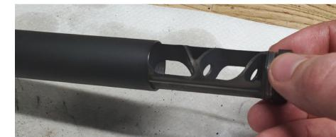
Insert the suppressor core, and thread into place. Torque the suppressor core only finger tight.
