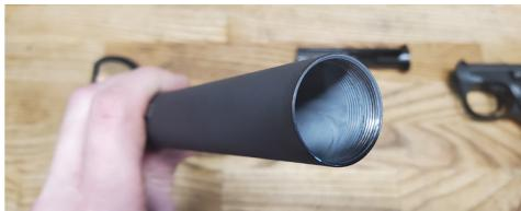
Clean deposits free using a rag or nylon brush with a solvent or oil.
