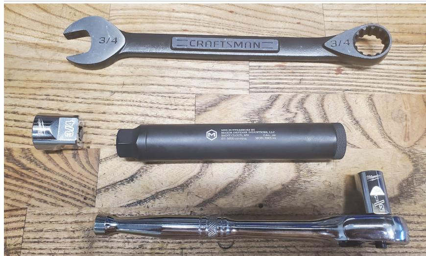
The suppressor tube is torqued to the mount and red (permanent) Loctite® is used to bind them together. If there is a problem, return the suppressor to the factory where experienced technicians can separate and replace these components.
