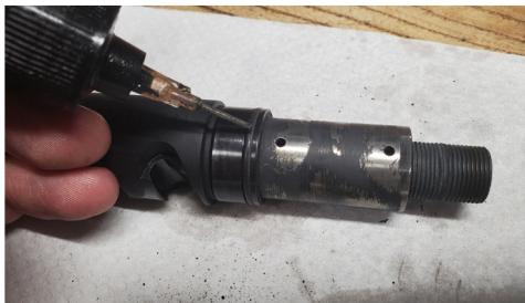
***CAUTION:** Be careful not to damage the O-ring. If the O-ring looks frayed or otherwise damaged, contact Maxim Defense Customer Service for a replacement.*
