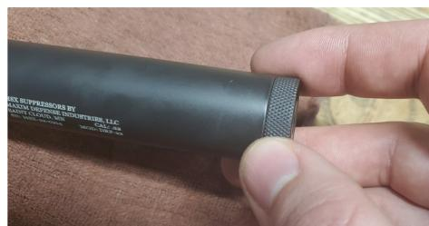
After maintenance has been conducted, reinsert the MonoKore into the tube and thread it back into place. The MonoKore should not be threaded tighter than finger tight using the knurled portion of the front of the MonoKore.
