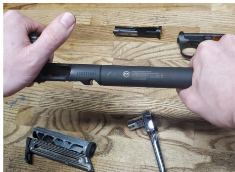
The suppressor tube is hand tight to the barrel. Unthread the suppressor tube from the receiver.
