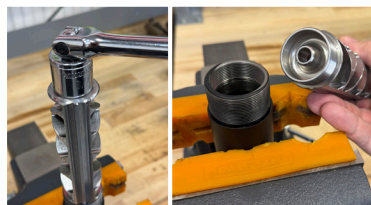
Typical build up areas are removed when the tube is removed.
